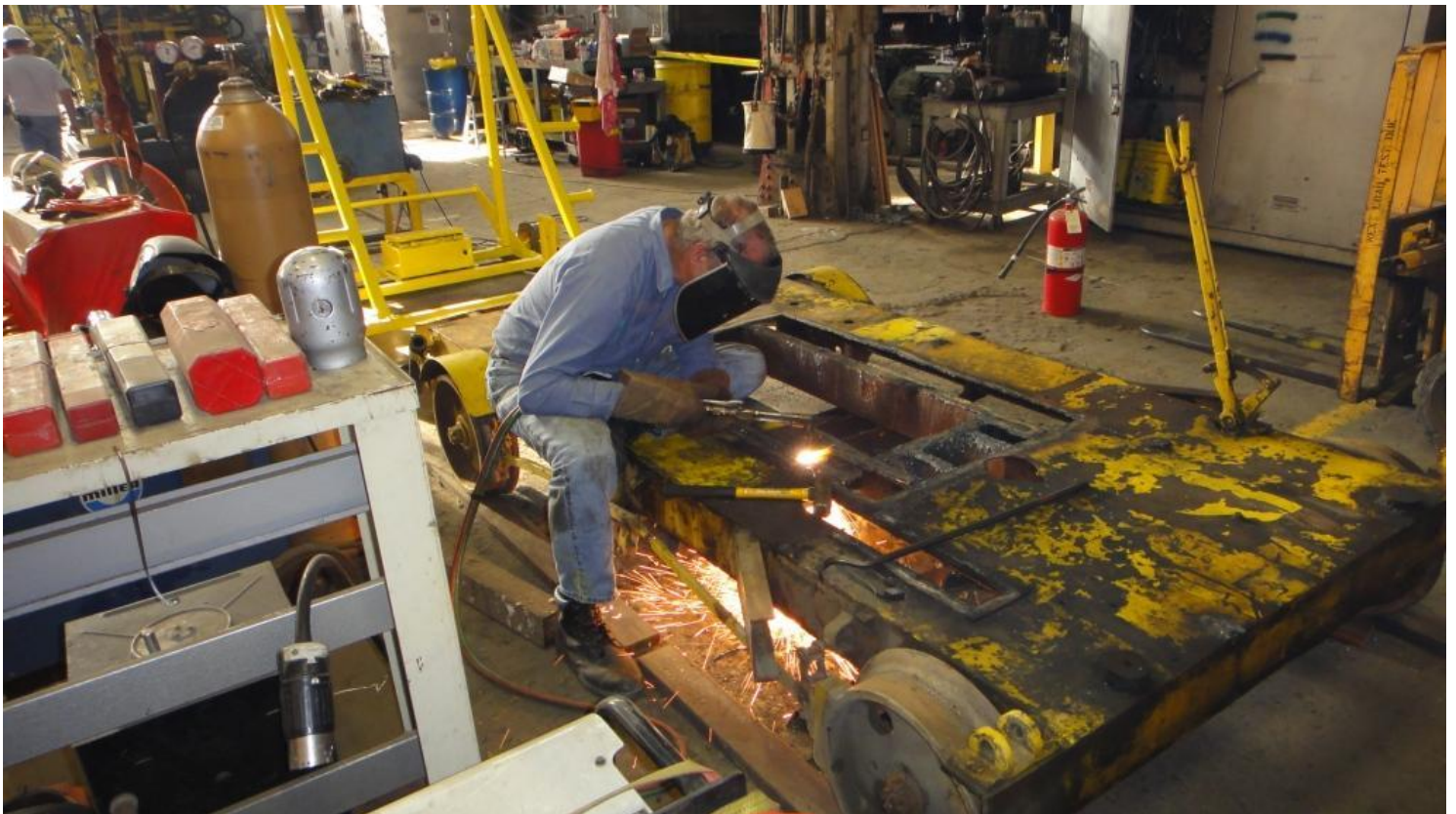
Alan cuts open the deck of the prehistoric tamper which is being converted to center-dump ballast hopper car
