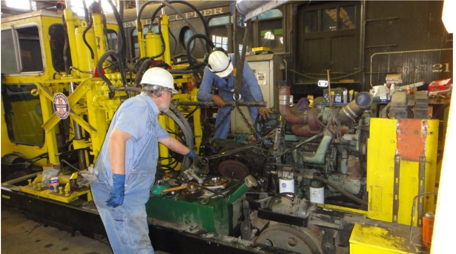
Bob and Fred removing the dual drive unit from the tie-shear which gave the Team access to the hydraulic pumps
